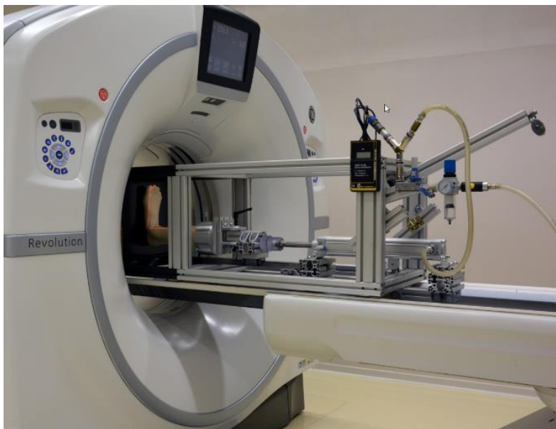
Figure 10.6.12: Custom-made, radiolucent, air pressure-controlled frame with a lower leg model mounted for CT scanning under axial loading.
