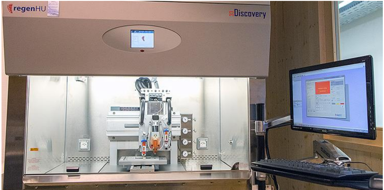
3-D Discovery Printer in a biosafety cabinet from regenHU Ltd. in the ARI.
