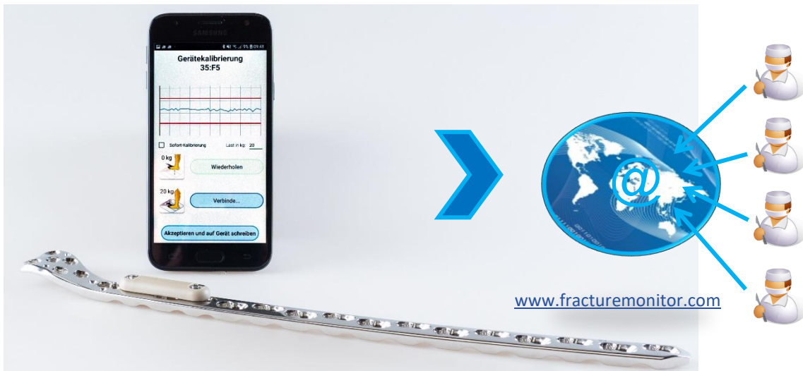
Figure 10.9.1: Illustration of the AO Fracture Monitor concept built around an implantable data logger allowing for remote assessment of fracture healing progression.
