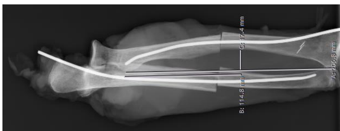
Figure 10.6.11: Anteroposterior radiograph of human cadaveric forearm with simulated AO PCCF 22-D/4.1 fracture, instrumented with 2 curved titanium elastic nails. Both implants left longer for easier explantation.
