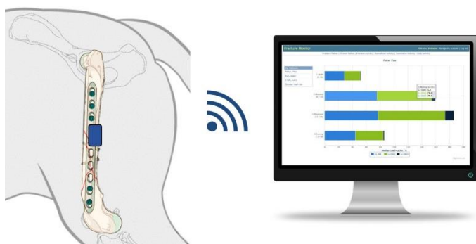
Figure 10.4.1: Implantable telemetric system with a sensor affixed to bone plate for continuous monitoring of healing progression in canine comminuted long bone fractures.
