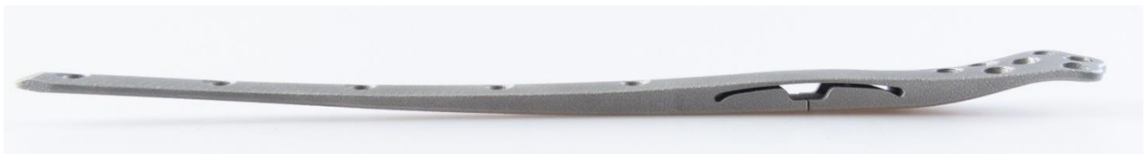
Figure 10.9.3: Rapid prototype of a biphasic distal femur plate produced with Selective Laser Sintering.
