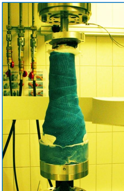
Figure 9.4.1: Biomechanical setup with an equine specimen mounted for testing.
