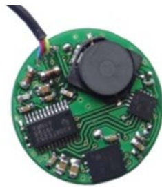
Data logger unit for on-board processing of in-vivo collected data.
