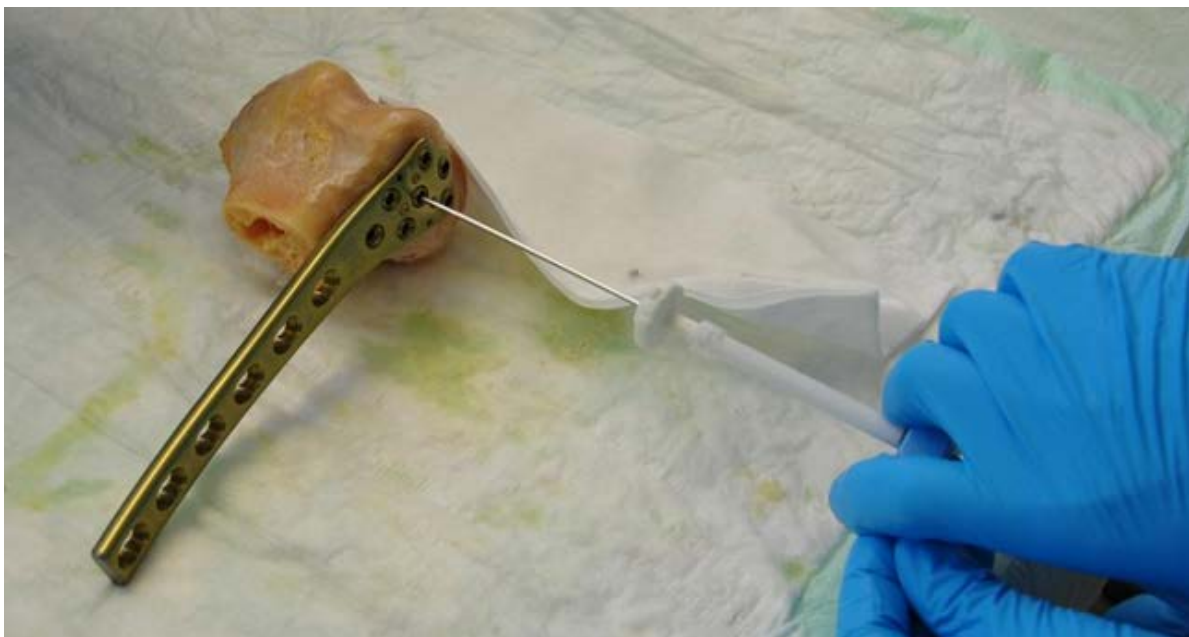
Injection of bone cement through cannulated screws in a human distal femur.
