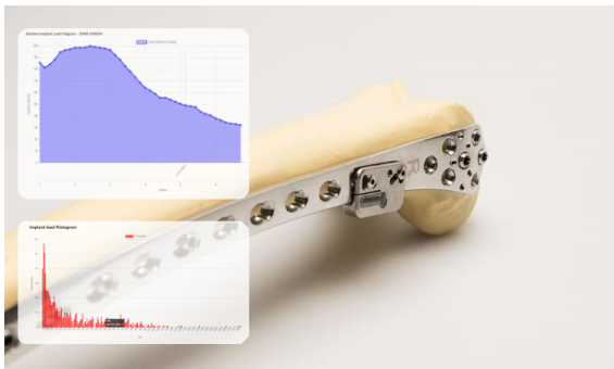
Figure 10.8.2: Implantable data logger attached to an LCP DF plate and exemplary data curves as provided in the cloud environment.
