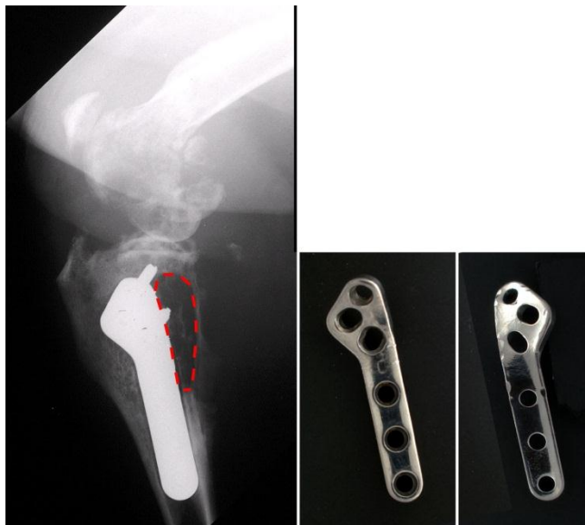
Radiograph of an operated dog knee with a large lysis zone (surrounded by a dotted line) in the tibia beneath the Slocum TPLO plate (left) and a contoured and explanted TPLO plate visualized from the bone (middle) and the soft tissue side (right).
